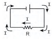
When more than one resistor is in a series circuit, the value of each resistor is added together to give the total resistance.
