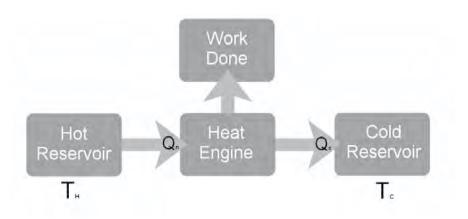
The flow chart above shows a generalized diagram of a heat engine. Heat from the hot reservoir  $(Q_h)$  flows from a high temperature area to a low temperature area. Between the two areas some of the heat energy is used to do work. The remaining heat  $(Q_c)$  becomes the exhaust.
