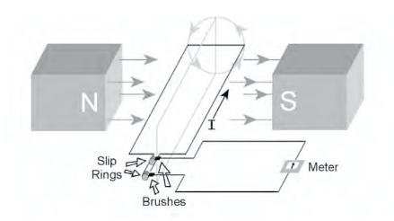
The current and voltage produced in the AC generators is not steady as in DC systems. Both current and voltage increase and decrease each time the loop of wire in the magnetic field turns a full 360°. The diagram below shows a comparison between AC and DC voltages.
