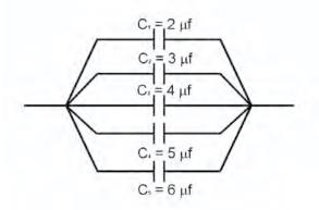
The six capacitors in the diagram have values of 2, 3, 4, 5, and 6 micro farads, respectively. The total capacitance is found by adding them together.
