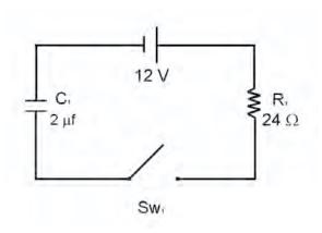
$C_1$  is an uncharged capacitor (shown in the circuit above). At t = 0 the switch (SW1) is closed, and  $C_1$  begins to charge.
