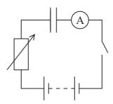
The capacitor is initially uncharged. When the switch is closed, there is a current in the circuit and the capacitor charges.
