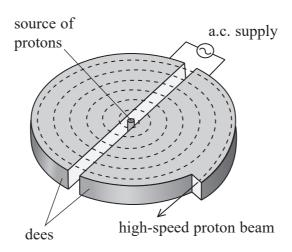
A magnetic field of uniform magnetic flux density B acts vertically upwards through the plane of the cyclotron. Protons travel along paths of increasing radius as their speed increases.
