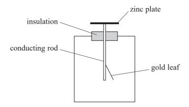
In a demonstration of the photoelectric effect, a teacher charged the zinc plate with a negative charge and the gold leaf was deflected.
