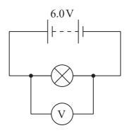
The voltmeter reading is 4.2 V.
