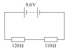
(i) Calculate the potential difference (p.d.) across the  $120\,\Omega$  resistor.
