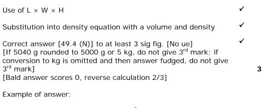
$80 \text{ cm} \times 50 \text{ cm} \times 1.8 \text{ cm} = 7200 \text{ cm}^3$   $7200 \text{ cm}^3 \times 0.70 \text{ g cm}^{-3} = 5040 \text{ g}$   $5040 \times 10^{-3} \text{ kg} \times 9.81 \text{ N/kg}$ = 49.4 N
