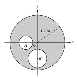
A uniform circular disc has centre O and radius 1.2 m. The centre of the disc is at the origin of x- and y-axes. Two circular holes with centres at A and B are made in the disc (see diagram). The point A is on the negative x-axis with OA = 0.5 m. The point B is on the negative y-axis with OB = 0.7 m. The hole with centre A has radius 0.3 m and the hole with centre B has radius 0.4 m. Find the distance of the centre of mass of the object from
