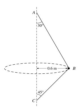
One end of a light inextensible string is attached to a fixed point A. The string passes through a smooth bead B of mass 0.3 kg and the other end of the string is attached to a fixed point C vertically below A. The bead B moves with constant speed in a horizontal circle of radius 0.6 m which has its centre between A and C. The string makes an angle of  $30^{\circ}$  with the vertical at A and an angle of  $45^{\circ}$  with the vertical at C (see diagram).
