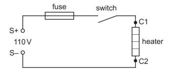
Terminals S+ and S- are the positive and negative terminals of the supply. Points C1 and C2 at either side of the heater are accessible for fault-finding.
