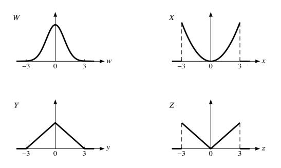
The diagrams show the probability density functions of four random variables W, X, Y and Z. Each of the four variables takes values between -3 and 3 only, and their standard deviations are  $\sigma_W$ ,  $\sigma_X$ ,  $\sigma_Y$  and  $\sigma_Z$  respectively.
