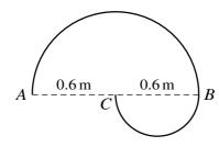
A uniform wire is bent to form an object which has a semicircular arc with diameter AB of length 1.2 m, with a smaller semicircular arc with diameter BC of length 0.6 m. The end C of the smaller arc is at the centre of the larger arc (see diagram). The two semicircular arcs of the wire are in the same plane.
