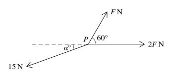
Three coplanar forces of magnitudes F N, 2F N and 15 N act at a point P, as shown in the diagram. Given that the forces are in equilibrium, find the values of F and  $\alpha$ . [6]
