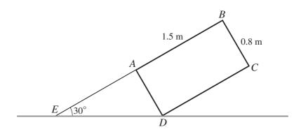
*ABCD* is the cross-section through the centre of mass of a uniform rectangular block of weight 260 N. The lengths *AB* and *BC* are 1.5 m and 0.8 m respectively. The block rests in equilibrium with the point *D* on a rough horizontal floor. Equilibrium is maintained by a light rope attached to the point *A* on the block and the point *E* on the floor. The points *E*, *A* and *B* lie in a straight line inclined at 30° to the horizontal (see diagram).
