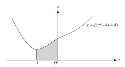
The diagram shows the curve  $y = \sqrt{(x^4 + 4x + 4)}$ .
