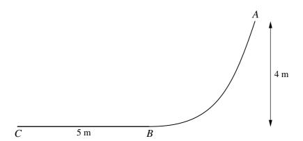
ABC is a vertical cross-section of a surface. The part of the surface containing AB is smooth and A is 4 m higher than B. The part of the surface containing BC is horizontal and the distance BC is 5 m (see diagram). A particle of mass  $0.8 \, \text{kg}$  is released from rest at A and slides along ABC. Find the speed of the particle at C in each of the following cases.
