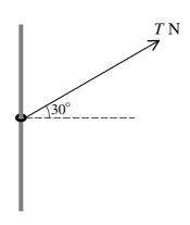
The diagram shows a ring of mass  $2 \, \text{kg}$  threaded on a fixed rough vertical rod. A light string is attached to the ring and is pulled upwards at an angle of  $30^{\circ}$  to the horizontal. The tension in the string is  $T \, \text{N}$ . The coefficient of friction between the ring and the rod is 0.24. Find the two values of  $T \, \text{for which the ring is in limiting equilibrium}$ .
