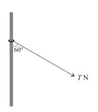
A ring of mass 4 kg is threaded on a fixed rough vertical rod. A light string is attached to the ring, and is pulled with a force of magnitude T N acting at an angle of 60° to the downward vertical (see diagram). The ring is in equilibrium.
