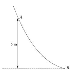
The diagram shows the vertical cross-section of a surface. *A* and *B* are two points on the cross-section, and *A* is 5 m higher than *B*. A particle of mass 0.35 kg passes through *A* with speed  $7 \text{ m s}^{-1}$ , moving on the surface towards *B*.
