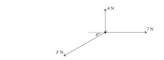
A particle is in equilibrium on a smooth horizontal table when acted on by the three horizontal forces shown in the diagram.
