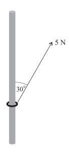
A small ring of mass  $0.6 \,\mathrm{kg}$  is threaded on a rough rod which is fixed vertically. The ring is in equilibrium, acted on by a force of magnitude 5 N pulling upwards at  $30^{\circ}$  to the vertical (see diagram).
