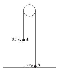
Two particles A and B, of masses 0.3 kg and 0.2 kg respectively, are attached to the ends of a light inextensible string which passes over a smooth fixed pulley. Particle B is held on the horizontal floor and particle A hangs in equilibrium. Particle B is released and each particle starts to move vertically with constant acceleration of magnitude a m s<sup>-2</sup>.
