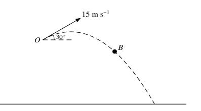
A small ball *B* is projected from a point *O* above horizontal ground, with initial speed  $15 \text{ m s}^{-1}$  at an angle of projection of  $30^{\circ}$  above the horizontal (see diagram). The ball strikes the ground 3 s after projection.
