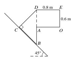
The diagram shows the cross-section *OABCDE* through the centre of mass of a uniform prism on a rough inclined plane. The portion *ADEO* is a rectangle in which AD = OE = 0.6 m and DE = AO = 0.8 m; the portion *BCD* is an isosceles triangle in which angle *BCD* is a right angle, and *A* is the mid-point of *BD*. The plane is inclined at 45° to the horizontal, *BC* lies along a line of greatest slope of the plane and *DE* is horizontal.
