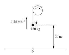
A load of mass  $160 \,\mathrm{kg}$  is pulled vertically upwards, from rest at a fixed point O on the ground, using a winding drum. The load passes through a point A,  $20 \,\mathrm{m}$  above O, with a speed of  $1.25 \,\mathrm{m\,s^{-1}}$  (see diagram). Find, for the motion from O to A,
