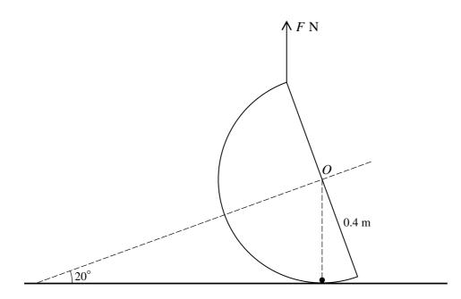
A smooth hemispherical shell, with centre O, weight 12 N and radius 0.4 m, rests on a horizontal plane. A particle of weight W N lies at rest on the inner surface of the hemisphere vertically below O. A force of magnitude F N acting vertically upwards is applied to the highest point of the hemisphere, which is in equilibrium with its axis of symmetry inclined at  $20^{\circ}$  to the horizontal (see diagram).
