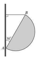
AB is the diameter of a uniform semicircular lamina which has radius 0.3 m and mass 0.4 kg. The lamina is hinged to a vertical wall at A with AB inclined at 30° to the vertical. One end of a light inextensible string is attached to the lamina at B and the other end of the string is attached to the wall vertically above A. The lamina is in equilibrium in a vertical plane perpendicular to the wall with the string horizontal (see diagram).
