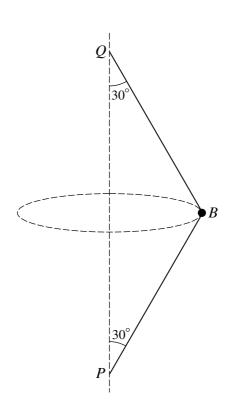
A small ball *B* of mass 0.4 kg is attached to fixed points *P* and *Q* on a vertical axis by two light inextensible strings of equal length. Both strings are taut and each is inclined at  $30^{\circ}$  to the vertical. The ball moves in a horizontal circle (see diagram).
