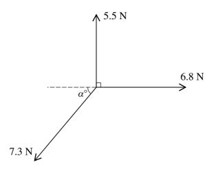
Three coplanar forces act at a point. The magnitudes of the forces are 5.5 N, 6.8 N and 7.3 N, and the directions in which the forces act are as shown in the diagram. Given that the resultant of the three forces is in the same direction as the force of magnitude 6.8 N, find the value of  $\alpha$  and the magnitude of the resultant.
