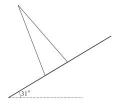
The cone is placed with its axis vertical on a rough horizontal plane. The plane is slowly tilted, and the cone remains in equilibrium until the angle of inclination of the plane reaches  $31^{\circ}$  (see diagram), when the cone topples.
