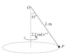
A particle *P* of mass *m*kg is attached to one end of a light inextensible string of length *L*m. The other end of the string is attached to a fixed point *O*. The particle *P* moves with constant speed in a horizontal circle, with the string taut and inclined at 35° to the vertical. *OP* rotates with angular speed 2.2 rad s<sup>-1</sup> about the vertical axis through *O* (see diagram). Find
