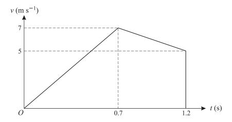
The diagram shows the velocity-time graph for the motion of a small stone which falls vertically from rest at a point A above the surface of liquid in a container. The downward velocity of the stone t s after leaving A is v m s<sup>-1</sup>. The stone hits the surface of the liquid with velocity 7 m s<sup>-1</sup> when t = 0.7. It reaches the bottom of the container with velocity 5 m s<sup>-1</sup> when t = 1.2.
