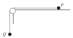
Particles P and Q are attached to opposite ends of a light inextensible string. P is at rest on a rough horizontal table. The string passes over a small smooth pulley which is fixed at the edge of the table. Q hangs vertically below the pulley (see diagram). The force exerted on the string by the pulley has magnitude  $4\sqrt{2}$  N. The coefficient of friction between P and the table is 0.8.
