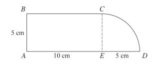
A uniform lamina *ABCDE* consists of a rectangular part with sides 5 cm and 10 cm, and a part in the form of a quarter of a circle of radius 5 cm, as shown in the diagram.
