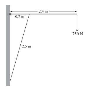
A uniform beam has length 2.4 m and weight 68 N. The beam is hinged at a fixed point of a vertical wall, and held in a horizontal position by a light rod of length 2.5 m. One end of the rod is attached to the beam at a point 0.7 m from the wall, and the other end of the rod is attached to the wall at a point vertically below the hinge. The beam carries a load of 750 N at its end (see diagram).
