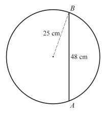
A frame consists of a uniform circular ring of radius  $25 \,\mathrm{cm}$  and mass  $1.5 \,\mathrm{kg}$ , and a uniform rod of length  $48 \,\mathrm{cm}$  and mass  $0.6 \,\mathrm{kg}$ . The ends A and B of the rod are attached to points on the circumference of the ring, as shown in the diagram. Find the distance of the centre of mass of the frame from the centre of the ring.
