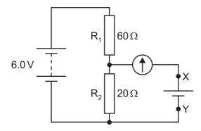
The circuit is to be used to test whether the electromotive force (e.m.f.) of a particular cell is 1.5 V. The cell is connected between terminals X and Y in parallel with  $R_2$  and in series with a galvanometer.
