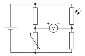
Which changes, if any, in temperature and light intensity would cause the voltmeter reading to decrease?
