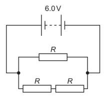
The total power dissipated in the resistor network is 24 W.
