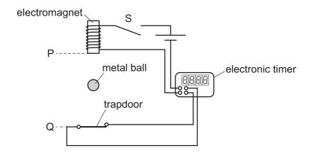
When switch S is opened, the ball is released from an electromagnet and an electronic timer is started. The ball then falls vertically downwards. The timer stops when the ball hits a trapdoor. The student measures the distance PQ between the electromagnet and the trapdoor. This distance and the reading on the timer are then used to calculate the acceleration of free fall.
