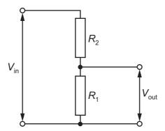
Which changes to  $R_1$  and  $R_2$  will increase the value of  $V_{out}$ ?
