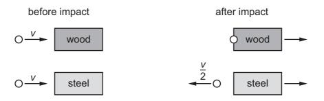
The wooden block and the steel block have equal mass.
