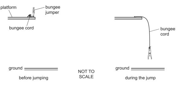
When the jumper makes the jump, his initial gravitational potential energy is converted into his kinetic energy and into elastic potential energy in the cord.
