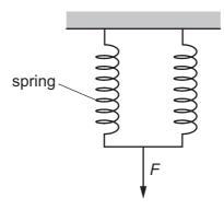
What is the extension and total elastic potential energy of this arrangement when the same force F is applied?
