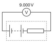
When a resistor of resistance  $11.0\Omega$  is connected in parallel with the battery, the voltmeter reading changes to 8.800 V.
