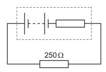
The current in the resistor is 40 mA for a time of 60 s. During this time 6.0 J of energy is dissipated by the internal resistance.
