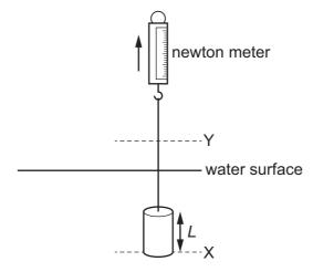
The cylinder, of height L, is slowly raised vertically by lifting the newton meter.
