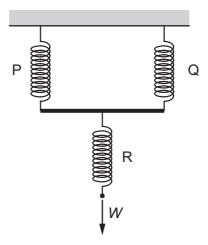
Springs P and Q are identical and each has spring constant k. Spring R has spring constant 3k.
