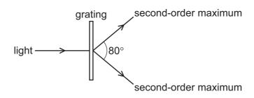
The angle between the second-order diffraction maxima is 80°, as shown.
