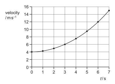
The vehicle, moving at  $4.0 \,\mathrm{m\,s^{-1}}$ , begins to accelerate at time t = 0.
