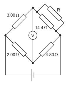
The reading on the voltmeter is zero.
