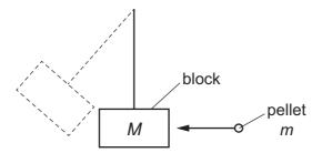
A pellet of mass m travelling at a speed u hits a stationary block of mass M. The pellet becomes embedded in the block and causes the block to move at a speed v immediately after the impact.
