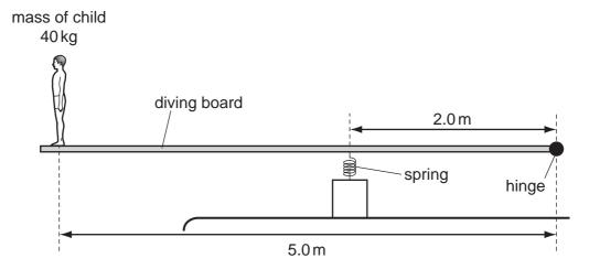
What is the extra compression of the spring caused by the child standing on the end of the board?
