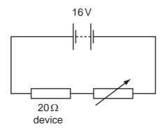
What is the resistance of the variable resistor when the power dissipated in the electrical device is 4.0 W?
