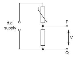
Which graph shows the variation with Celsius temperature  $\theta$  of potential difference V between points P and Q?
