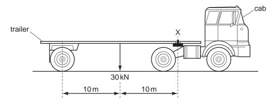
What is the upward force exerted by the cab on the trailer at X?
