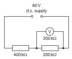
What is the reading on a voltmeter, also of resistance 200 k $\Omega$ , when connected across the 200 k $\Omega$  resistor as shown in the diagram?
