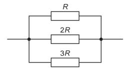
Using I to represent the current through the resistor of resistance R, which row represents the relationships between the currents through the resistors?
