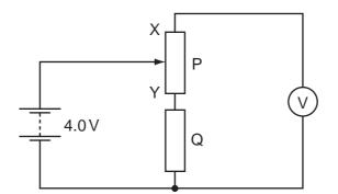
The slider on the potentiometer is moved from X to Y and a graph of voltmeter reading V is plotted against slider position.
