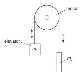
At what rate does the motor provide energy to the system when the elevator is rising at a steady speed v? (g = acceleration of free fall)
