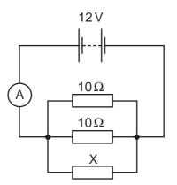
The battery has e.m.f. 12V and negligible internal resistance. The ammeter reading is 3.2A. What is the resistance of X?
