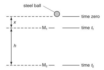
A steel ball is released at time zero from a point a distance x above M<sub>1</sub>. The ball reaches M<sub>1</sub> at time  $t_1$  and reaches  $M_2$  at time  $t_2$ . The acceleration of the ball is constant.
