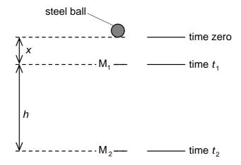
When a steel ball is released from rest from a point a distance x above M<sub>1</sub>, it is found that the ball takes time  $t_1$  to reach  $M_1$  and time  $t_2$  to reach  $M_2$ .
