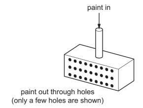
The paint is ejected at a speed of  $2.5 \,\mathrm{m\,s^{-1}}$  through 400 holes, each of area  $0.4 \,\mathrm{mm^2}$ . The density of the paint is  $900 \,\mathrm{kg\,m^{-3}}$ .
