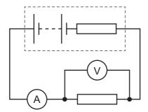
The battery is replaced by a different battery that has the same electromotive force (e.m.f.) but a greater internal resistance.
