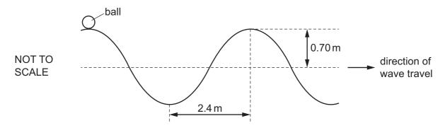
The wave has a frequency of 0.20 Hz and an amplitude of 0.70 m. The distance between a trough and an adjacent peak is 2.4 m.
