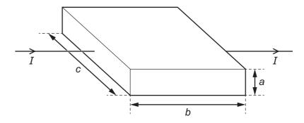
The block has sides of length a, b and c as shown, and its volume is V. Each charge carrier has a charge -q and the number density of the charge carriers in the metal is n. It takes each charge carrier an average time of *t* to pass through the block.
