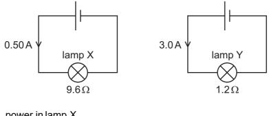
What is the ratio  $\frac{\text{power in lamp } X}{\text{power in lamp } Y}$ ?
