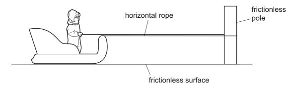
The rope is horizontal. The child pulls on the rope with a horizontal force of 12 N. This causes the child and the sledge to move with equal acceleration towards the pole.
