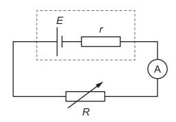
When *R* is  $10 \Omega$  the ammeter reads 0.3 A.
