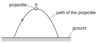
The projectile reaches its maximum height at position X. Assume that no upthrust acts on the projectile.
