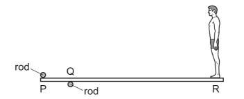
The forces exerted by the rods on the board are vertical. The board remains in equilibrium as the person slowly moves towards point Q from end R.
