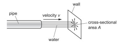
When the jet of water hits the wall, it has horizontal velocity v and cross-sectional area A.
