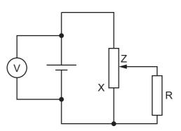
Which statement explains the change to the reading of the voltmeter as contact Z is moved towards end X of the potentiometer?
