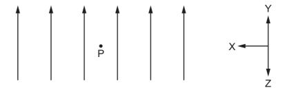
The field lines (lines of force) are evenly spaced and parallel.
