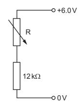
What is the resistance of the variable resistor R to give a potential difference of 1.0 V across the  $12 k\Omega$  resistor?
