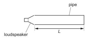
When a stationary wave is formed, there is an antinode at the open end of the pipe.
