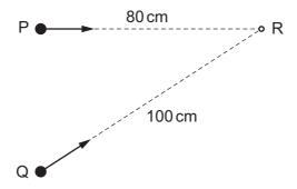
Both waves have a wavelength of 6.0 cm. The waves are in phase at point R.
