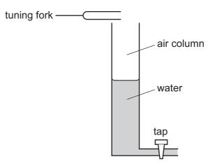
The tube is filled and then water is allowed to run out of it. The first two stationary waves occur when the air column lengths are 0.14 m and 0.42 m.
