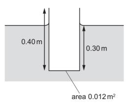
The cross-sectional area of the pipe is  $0.012 \text{ m}^2$ . The weight of the pipe is 32 N.
