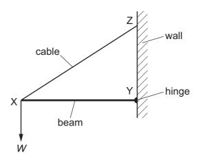
The beam supports a weight *W* at point X. The forces in the cable and the beam are  $F_{\rm C}$  and  $F_{\rm B}$  respectively.
