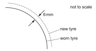
What is the error in the speed shown on the speedometer after this wear has taken place?
