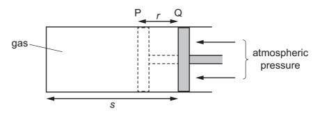
The gas is heated and this causes it to expand, pushing back the piston through distance r from position P to position Q. The length of the gas column is then s.
