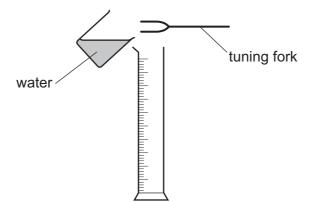
Water is then gradually poured into the measuring cylinder. A much louder sound is first heard when the water level is 2.9 cm above the base of the measuring cylinder. A second much louder sound is heard when the water level reaches a height of 67.3 cm above the base.
