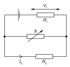
$V_1$  is the potential difference across the resistor of resistance  $R_1$ .
