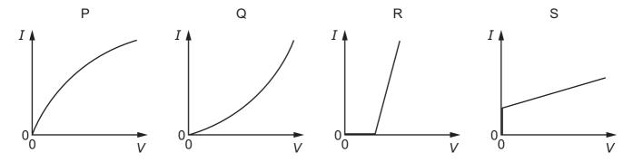
Which row in the table best specifies the correct *I-V* graphs for the lamp and for the diode?
