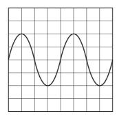
The setting of the time-base is then changed from  $10\,\mathrm{ms\,cm^{-1}}$  to  $20\,\mathrm{ms\,cm^{-1}}$  and the Y-plate sensitivity remains constant.
