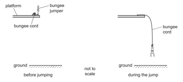
When the jumper makes the jump, his initial gravitational potential energy is converted into his kinetic energy and into elastic potential energy in the cord.
