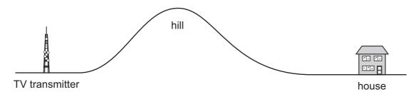
By which wave effect at the hill could the TV signal reach the house?
