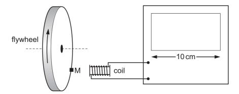
The flywheel has a small magnet M mounted on it. Each time the magnet passes the coil, a voltage pulse is generated, which is passed to the c.r.o. The display of the c.r.o. is 10 cm wide. The flywheel is rotating at 3000 revolutions per minute.
