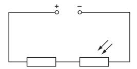
When the LDR is in the dark, the fixed resistor and the LDR have the same value of resistance.
