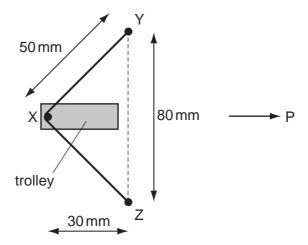
X is at the centre of the elastic and the trolley is to be propelled in the direction P at right angles to YZ. The tension in the elastic is 4 N.
