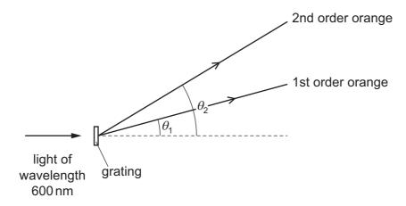
What is the angular separation  $(\theta_2 - \theta_1)$  between the first and second order maxima of the orange light?
