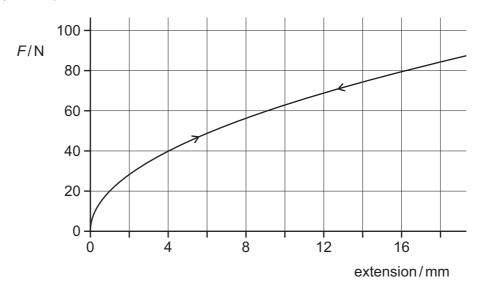
What is the best estimate of the strain energy in the rubber when a load of 80 N is applied?
