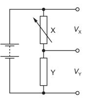
The potential difference across resistor X is  $V_X$  and the potential difference of resistor Y is  $V_Y$ .
