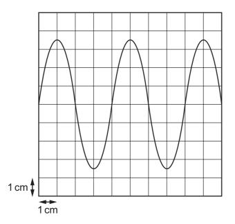
The oscilloscope time-base setting is  $0.5 \,\mathrm{ms}\,\mathrm{cm}^{-1}$  and the Y-plate sensitivity is  $2 \,\mathrm{V}\,\mathrm{cm}^{-1}$ .
