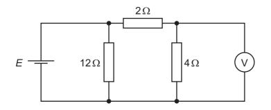
The voltmeter has a very high resistance and reads a potential difference  $V_{out}$ .
